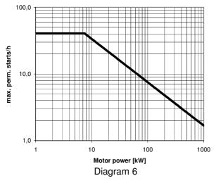
With electric motors, the permitted number of starts is given in the attached motor operating instructions. If two different figures are given, the lower figure is valid.
