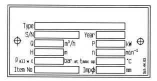
Type \*) Type of pump S/N \*) Serial number Year Year of construction
