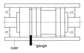
pic 5 - Alignment of coupling with spacer
