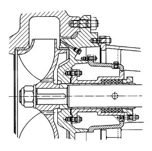
Design LS, LC, LCP Stuffing box with cooling jacket for temperatures up to 180°C (350°F)
