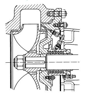
Design LS, LC, LCP Stuffing box optional with internal or external flush for temperatures up to 140°C (280°F)
